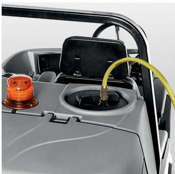
A simple device allows the quick filling of the tank with clean water without the presence of the operator
