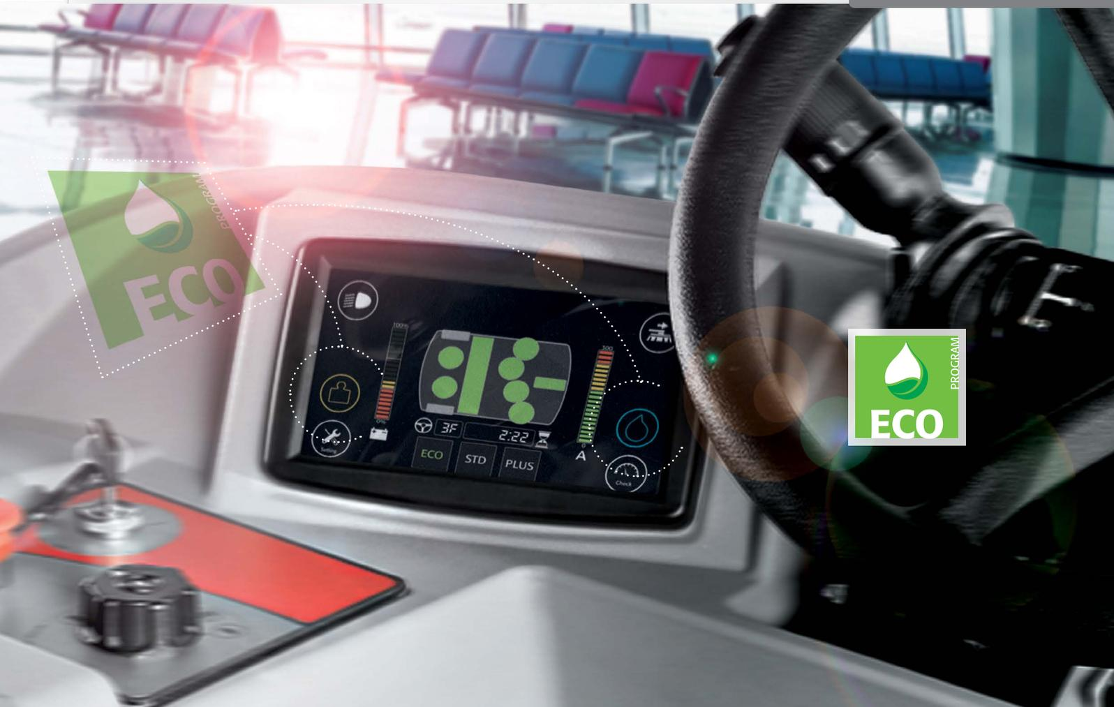
The C130 uses technologies that help save resources. Indeed, when running cleaning operations in ECO mode, the supply of water, detergent and pressure is reduced to a minimum.
