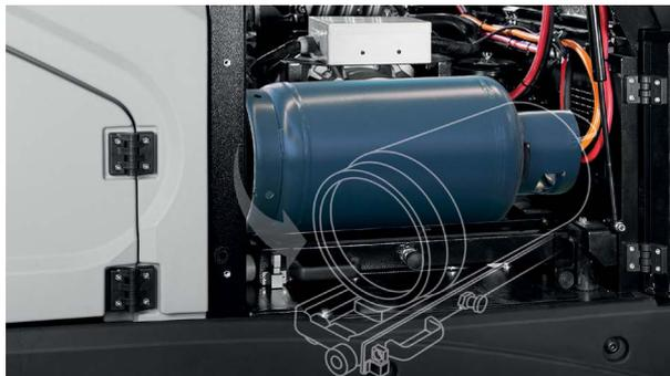
The engine area is easily accessible. In the bi-fuel version, a specific compartment has been created to house the LPG cylinder. The cylinder can be removed via a convenient stand that rotates towards the outside.
