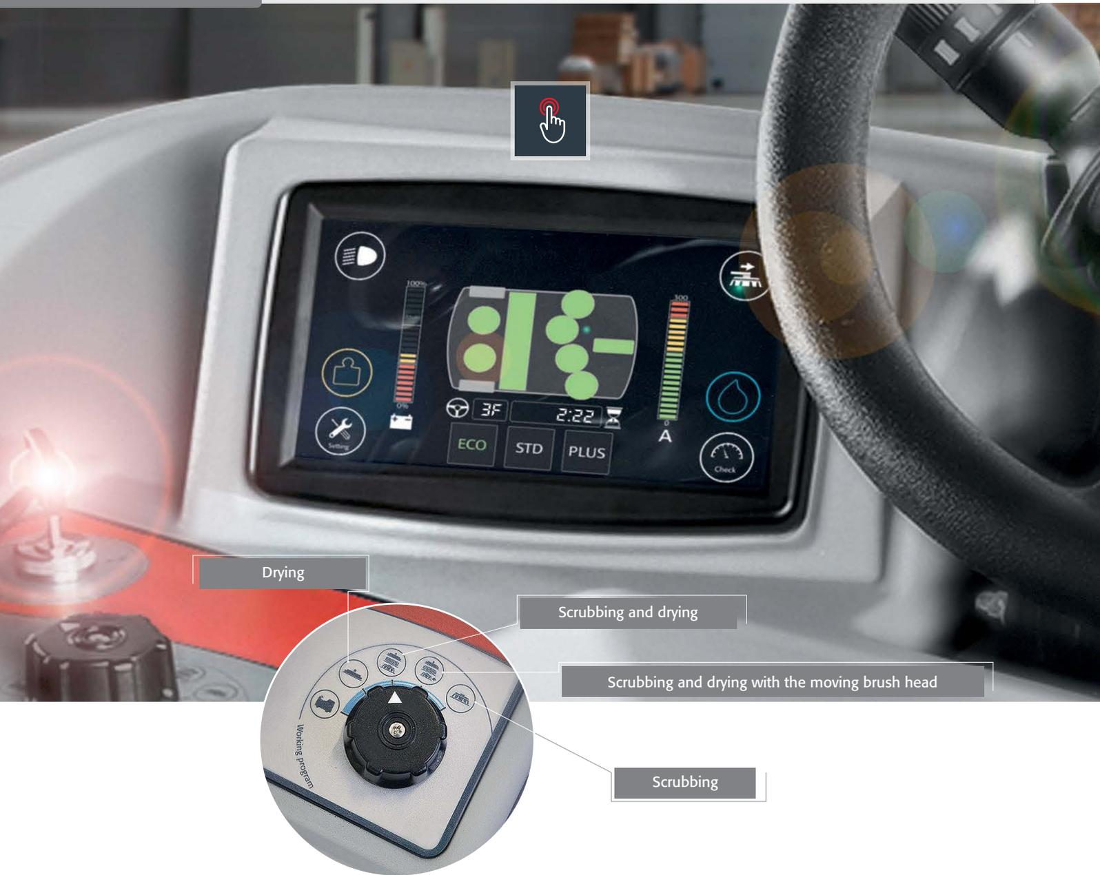
Using the C130 is simple, intuitive and practical. The working program selector enables the operator to manually select the type of activity to be carried out: scrubbing and drying, scrubbing and drying with the moving brush head, scrubbing only, or drying only.
