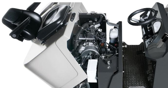
The opening gives complete accessibility to the components. Just the checking of the oil or changing the filters for instance, in the motorised version, is now very easy.
