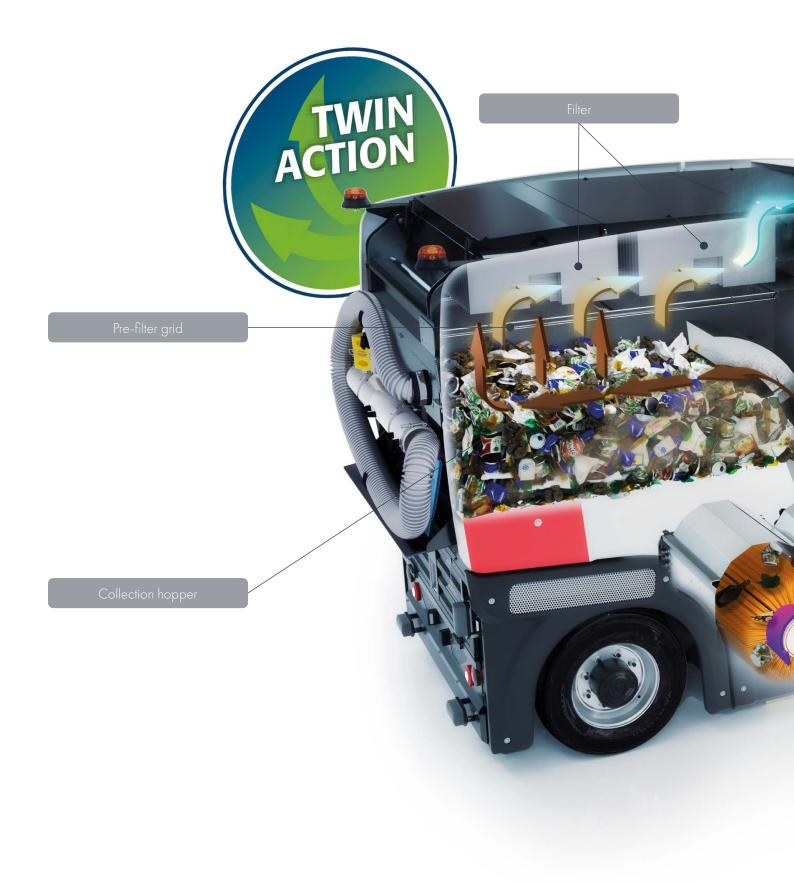
TwinAction is an exclusive technology, designed by Comac to allow the side brushes to move the material to be collected to the centre towards the central brush. This then in turn, thanks to the force of the mechanical action, collects the dirt from the ground and directs it towards a rotating shaft equipped with hammers capable of shredding and grinding the debris.
