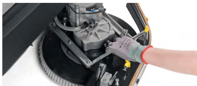
The brush head can be extracted on the left-hand side to facilitate the inspection and replacement of the central disc brush.
