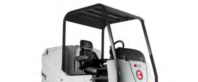
Possibility to install the overhead guard to protect the operator.
