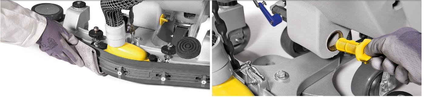
To ensure a perfect drying, the suction hose and the squeegee rubber blades must be cleaned at the end of any cleaning operation. The squeegee can be lifted to quickly clean the rubber blades.
