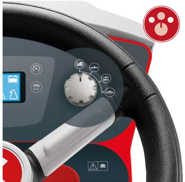
The automatic version is equipped with a **working program selector** making the use of the machine extremely intuitive. It allows to choose the selection of four pre-set working programs: Transfer, Drying, Scrubbing/Drying, Scrubbing only.
